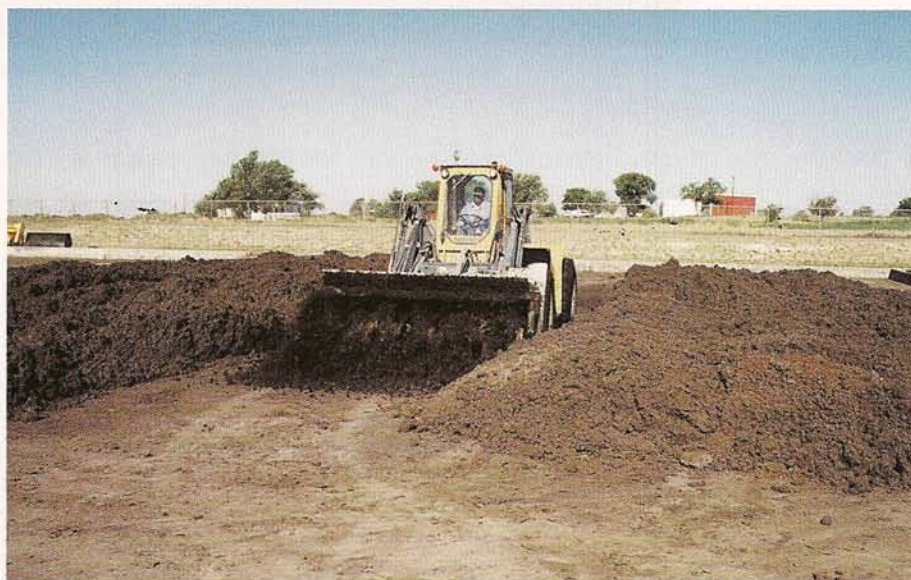
Biosolids are aerated in windrows.
